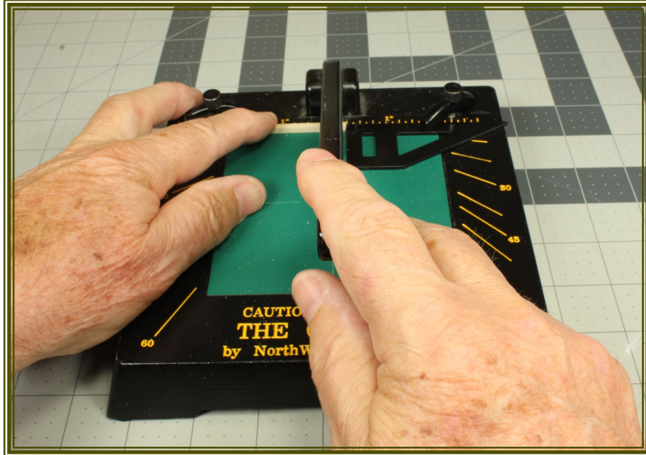
Figure 5 - Repeating cuts are possible using one of the supplied angle-stops. They clamp easily using the built-in thumb screws.
