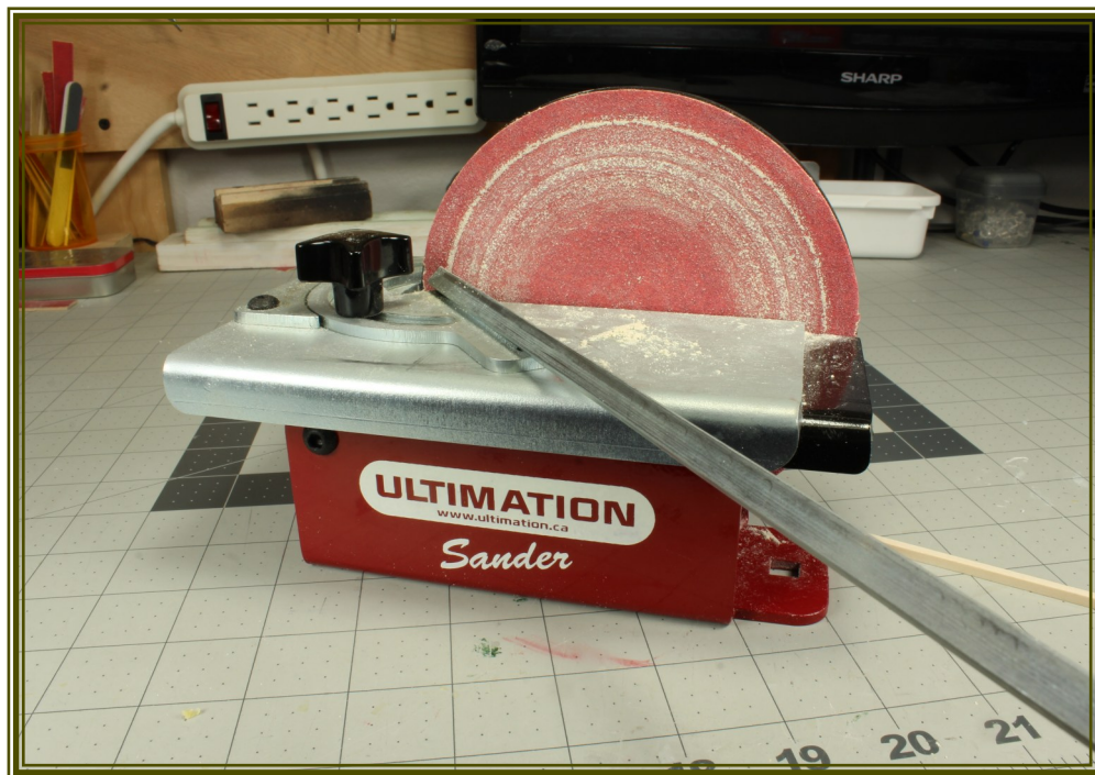
Figure 6 - By far this is the most expensive non-powered tool I own. It can be mounted to the workbench with bolts or a C-clamp. The repeater attachment is the long metal bar sticking out towards the camera.
