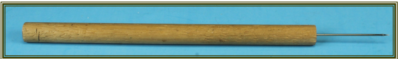
Figure 6 - A needle inserted into a wood dowel is a great tool to make nail holes.
