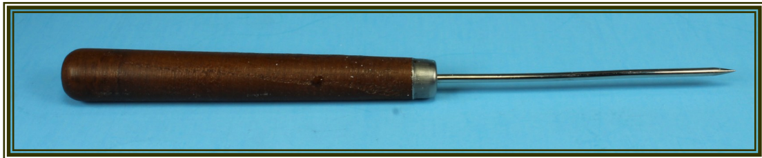
Figure 2 - This is the largest of the pointy tools on my workbench. I use it to start holes in pine lumber and other applications where I need to push hard.
