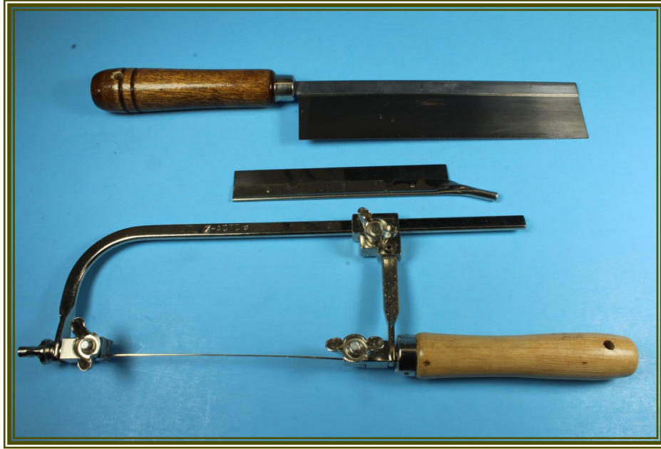
Figure 5 - Hobby saws shown: A fine-toothed razor saw with a solid wood handle, an old razor saw blade used for scraping texture into wood and styrene, and a jeweler's saw for curved cuts.
