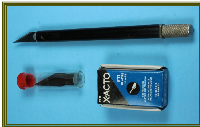
Figure 2 - The No 11 blade is THE blade we all use. I buy them in bulk but move a few to a clear container I keep handy.
