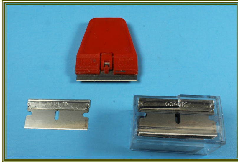
Figure 3 - Single edge razor blades continue to be a key cutting tool. An inexpensive window scraper provides a safe and effective handle.
