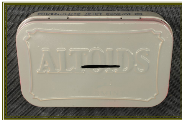
Figure 4 - A slot cut in an old mint tin serves as a container for used blades. I sprayed it gray, so I won't confuse it with my mints!
