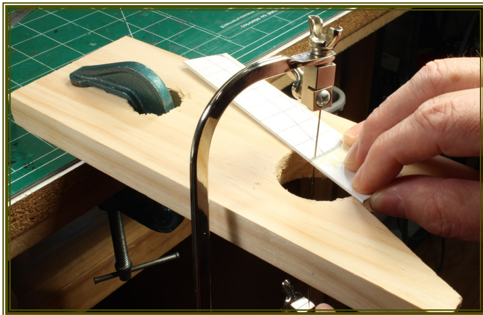
Figure 6 - A piece of scrap wood was fabricated into an effective extension to the workbench and allows me to make intricate cuts with a jeweler's saw.
