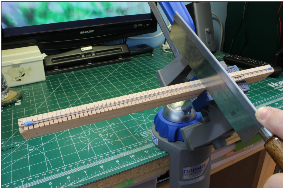
1 - Cutting wooden shingle strips using a fixture, hobby vise and razor saw
