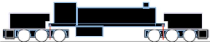
The principal benefit of the Garratt design is that the boiler and firebox unit are slung between the two engine units. This frees the boiler and the firebox from the size constraints imposed where they are placed over the frames and running gear.
